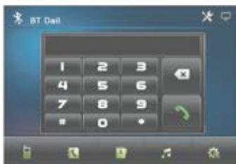
2. Make a phone call from the car radio by entering the number to call using the numeric buttons on the remote control or directly on the LCD screen.
